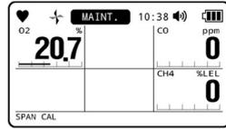
Span adjustment is performed.
