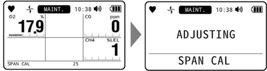
The following results are displayed when the bump test and gas adjustment have ended. Press the ▲/AIR or RESET/▼ button to toggle the results display.
