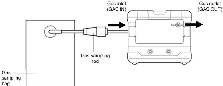
**<When using the CF-284 CO<sub>2</sub> removal filter>**
