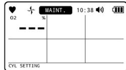
5 Press the ▲/AIR or RESET/▼ button to set the sensor, then press the POWER/ENTER button. Press the button repeatedly to cycle through the following settings [A] → [B] → [C] ... [F]. Note that cylinders that cannot be set will not be displayed.
