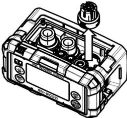
For the F sensor, remove the sensor.
