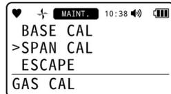
3 Press the ▲/AIR or RESET/▼ button to select the cylinder to be adjusted, then press the POWER/ENTER button.
