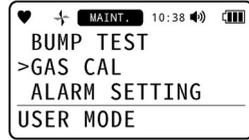
2 Press the ▲/AIR or RESET/▼ button in the [GAS CAL] menu to select [SPAN CAL], then press the POWER/ENTER button.
