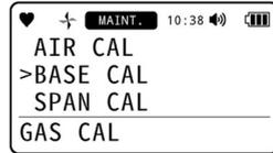
3 Introduce the base gas adjustment gas, wait 120 seconds, then press the POWER/ENTER button. For the gas type used for base gas adjustment, use the gas (nitrogen (N<sub>2</sub>) or inert gas) selected for [TE BASE SELECT] in user mode.
